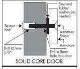
Drill an 8mm hole thru door. From sexnut bolt side of door, drill 12.7mm (1/2") hole, 25mm (1") in depth.
